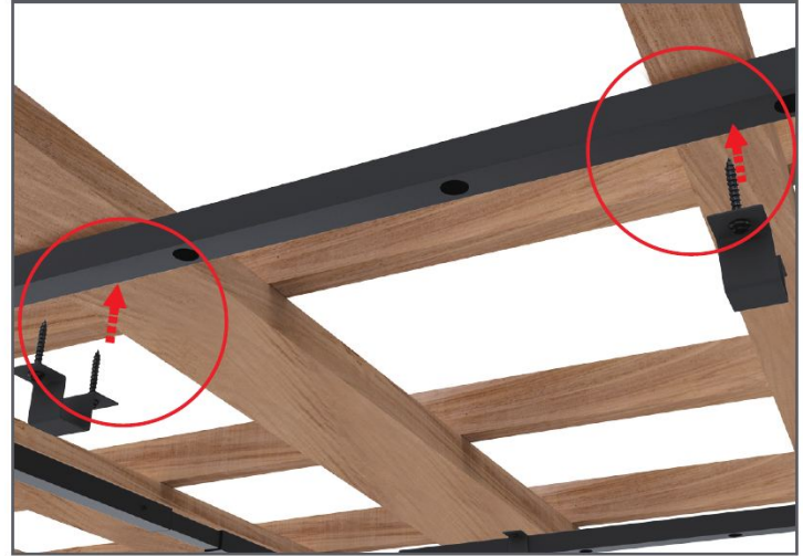
B: Secure the ceiling brackets onto the supporting wood using U-Clamps N and Hex Head Lag Screws P .
